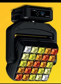
With 900 W of total power, the versatile MagicPanel FX has 25 next-generation RGBW high-power LED emitters and an active phase-change liquid cooling system using a heat pipe for intensive use in "wash light" mode. The continuous, unlimited, rotation on pan and tilt, first introduced on the legendary MAGICPANEL 602 in 2013, is standard. MAGICPANEL FX has serial connectivity and can be controlled using DMX-RDM, ArtNet™, sACN or wireless CRMX TiMo RDM by LumenRadio™.
